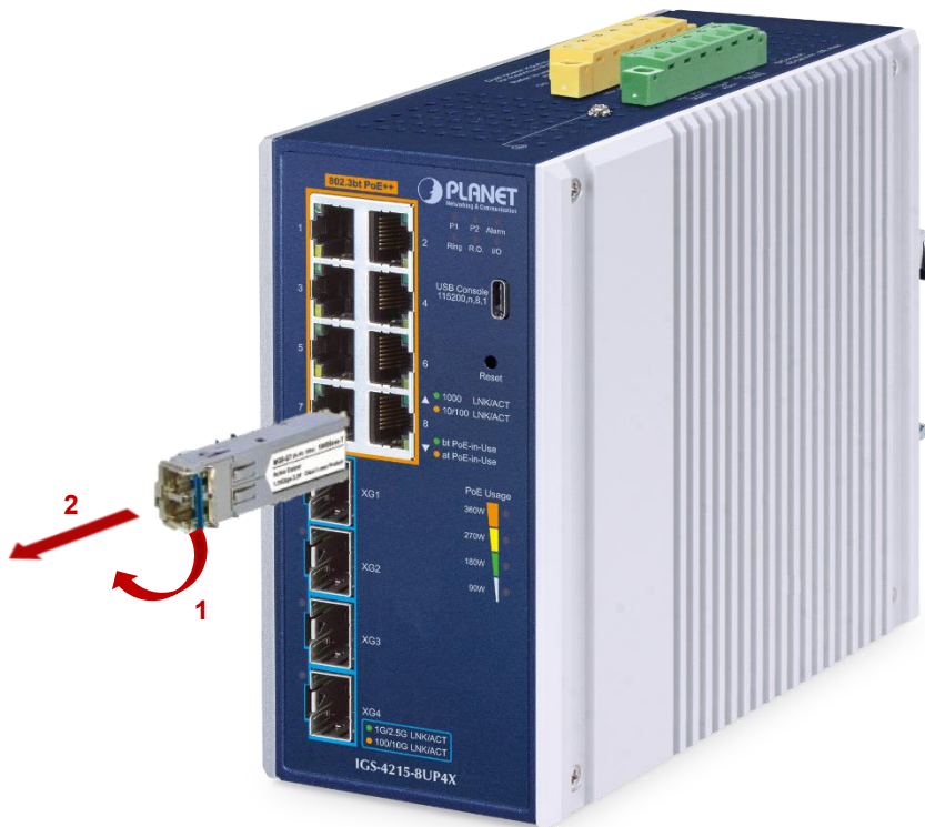
Figure 2-2-5: Remove the SFP Transceiver Module
