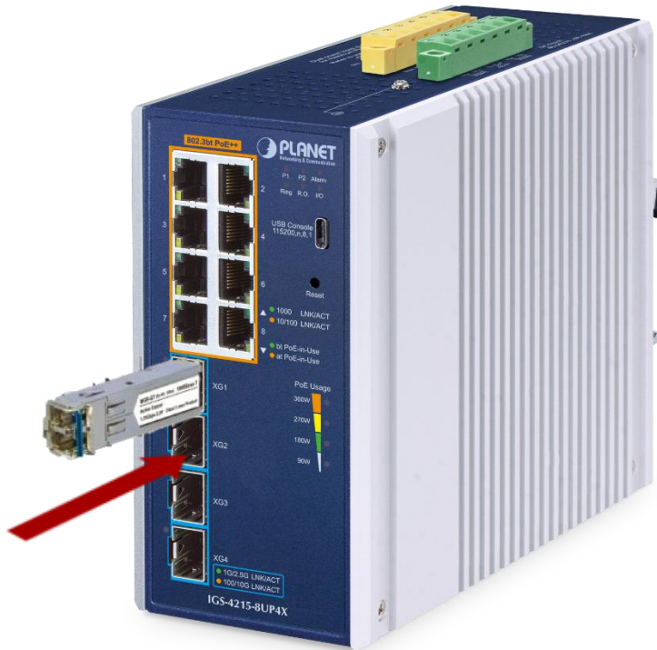
Figure 2-2-4: Plug in the SFP Transceiver
